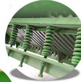
Yaylı Elek Sistemi Screen system with spring
